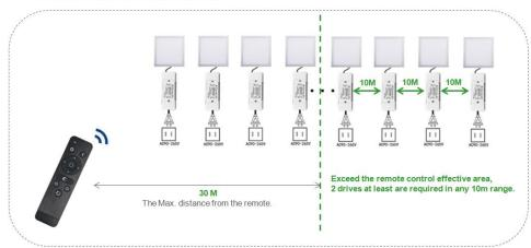
Range of control on 2.4G Smart system is not limited from the range of remote controller. In a large premises, exceeding the range of remote controller, drivers/dimers transmits signal among themselves and inspect the light state for each other. This is possible when distance between drivers/dimers is less than 10 meters.
